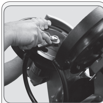
Hold wheel while loosening bolts.
