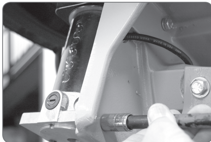
Figure 8 Shown using a 6" extension with 7/16" socket.
