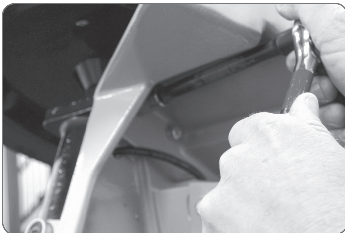
Figure 7 Shown using a 6" extension with 1/2" socket.
