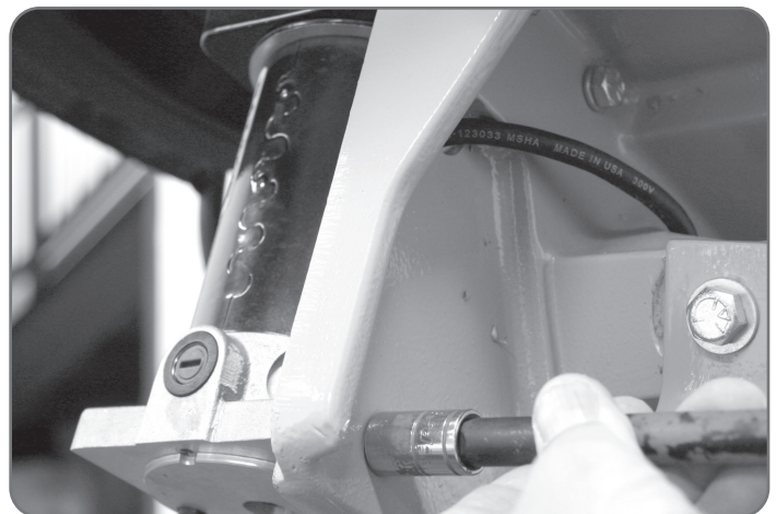
Figure 8 Shown using a 6" extension with 7/16" socket.
