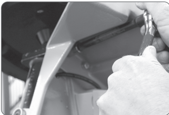
Figure 7 Shown using a 6" extension with 1/2" socket.
