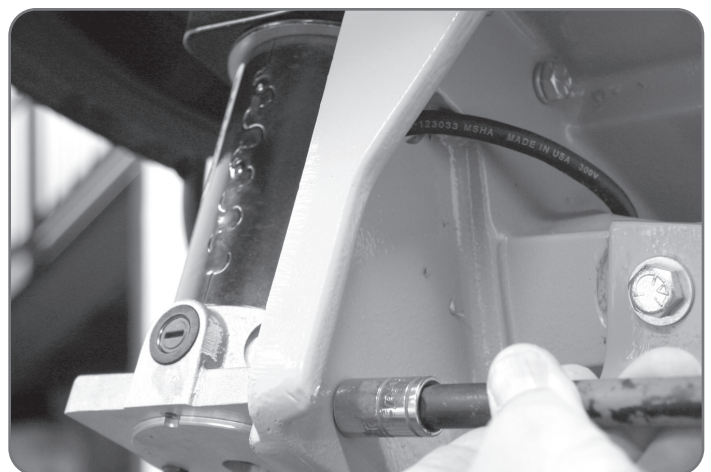
Figure 17 Shown using a 6" extension with \frac{7}{16} " socket.
