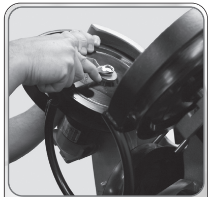
Hold wheel while loosening bolts.
