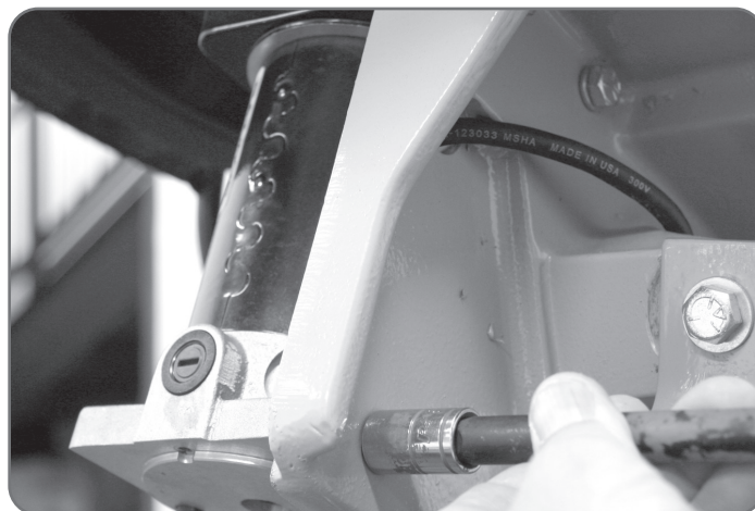
Figure 10 Shown using a 6" extension with 7/16" socket.
