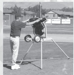
Figure 4 Carefully tilt Junior Softball Hack Attack up onto its rear legs.
