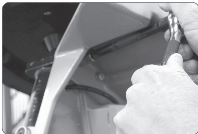
Figure 9 Shown using a 6" extension with 1/2" socket.
