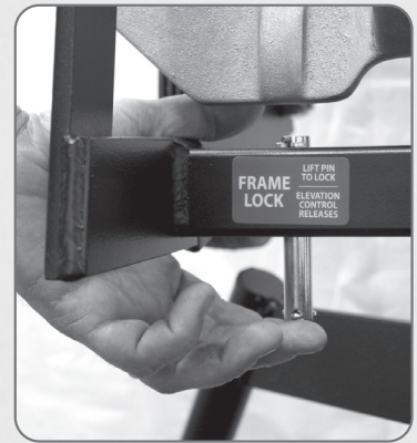
Figure 8A Push up frame lock pin.
