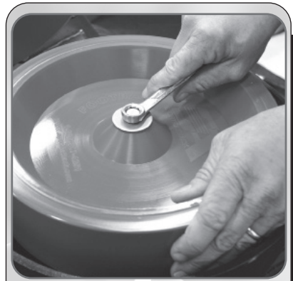
Figure 8 Hold wheel in place while loosening bolts.
