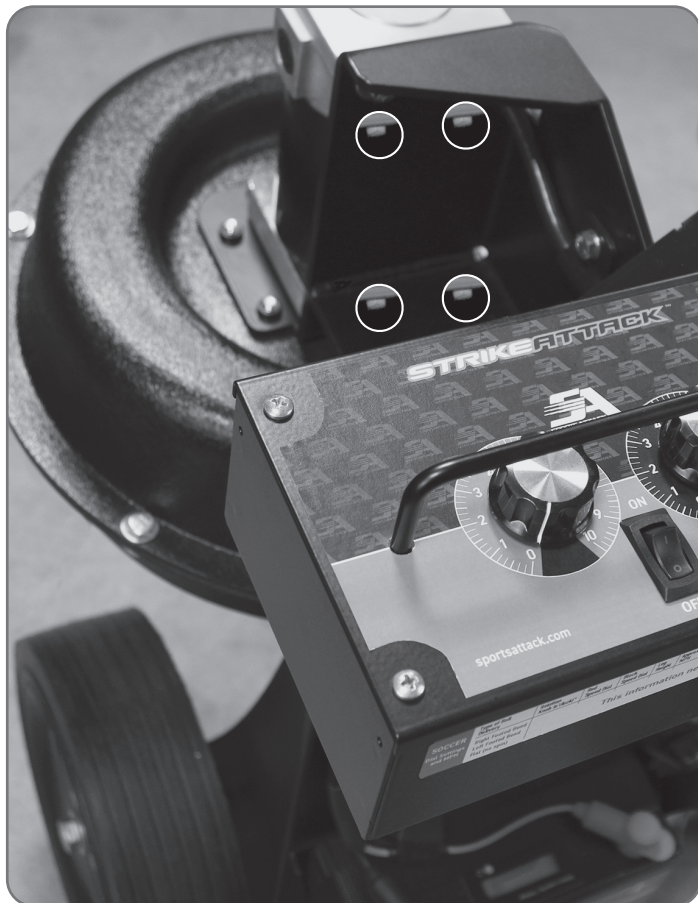
Figure 2 Showing the four bolts to unbolt for removing the motor.
