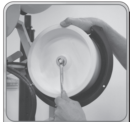
Figure 9 Hold wheel while loosening bolts.
