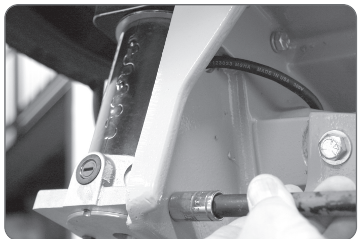
Figure 17 Shown using a 6" extension with 7/16" socket.
