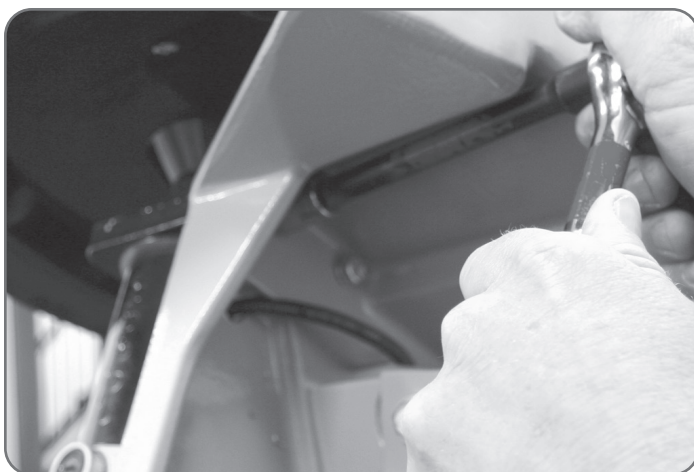
Figure 16 Shown using a 6" extension with 1/2" socket.
