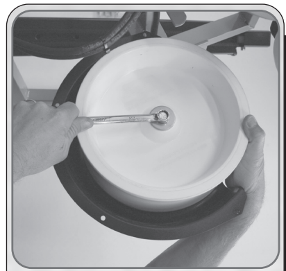
Figure 1 Hold the wheel while loosening bolts with a half inch box-end wrench.
