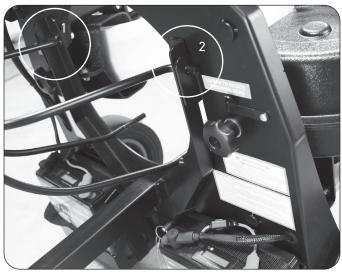
**Detail A** Install Chute/Handle Assembly onto main frame of Strike Attack machine as follows: Place 90 degree tabs on chute/handle over hooks on either side of ball tunnel and slide bottom of Chute/Handle assembly into retaining slot.
