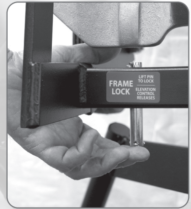
Figure 8A Push up frame lock pin
