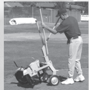
Figure 2 Tip up onto wheel guard; Insert two front legs
