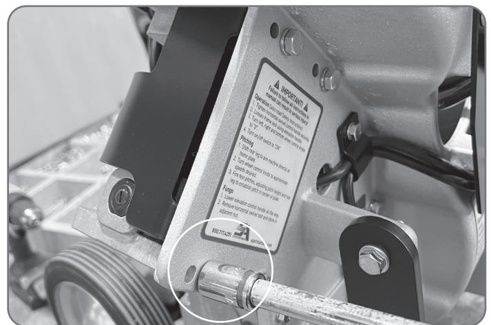
Figure 10 Shown using a 6" extension with 7/16" socket.
