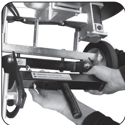
Figure 6 Attaching throwing head to undercarriage.
