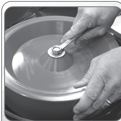
Figure 10 Hold wheel in place while loosening bolts.
