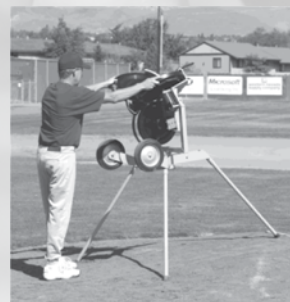
Figure 4 Carefully tilt I-Hack Attack up onto its legs
