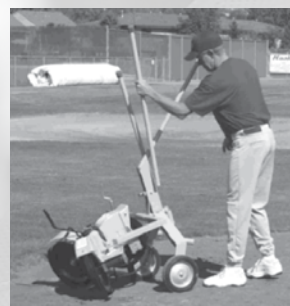
Figure 2 Tip up onto wheel guard; Insert two front legs
