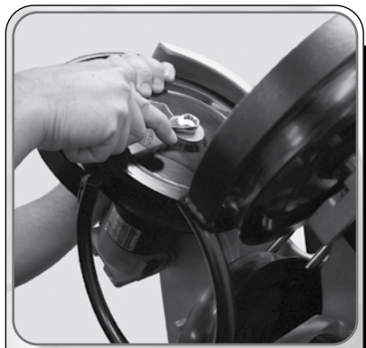
Hold wheel while loosening bolts.
