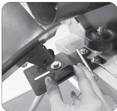
Figure 5B Align ball feed tray from Team Ball Feeder to pitching machine (Side View).
