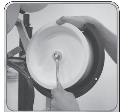
Figure 9 Hold wheel while loosening bolts.
