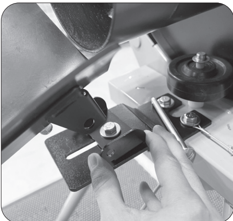
Figure 5B Align ball feed tray from Elite Team Ball Feeder to pitching machine (Side View).
