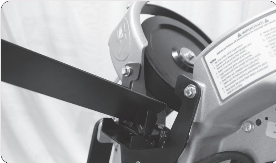
Figure 9 Ball tray assembly at pitching machine with mounting bracket (ball tray to feeder) installed.
