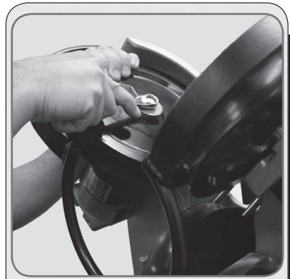
Hold wheel while loosening bolts.
