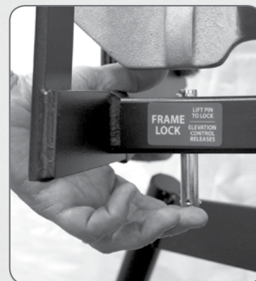
Figure 8A Push up frame lock pin.
