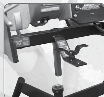
Figure 8D Lift the throwing head completely out of the undercarriage.
