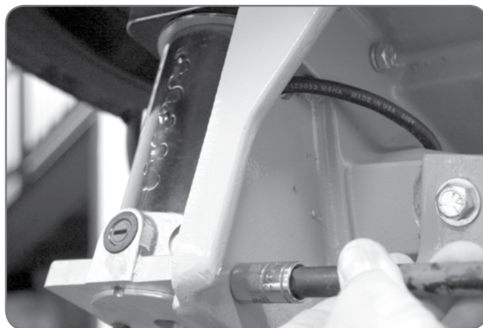
Figure 10 Shown using a 6" extension with \frac{7}{16} " socket.
