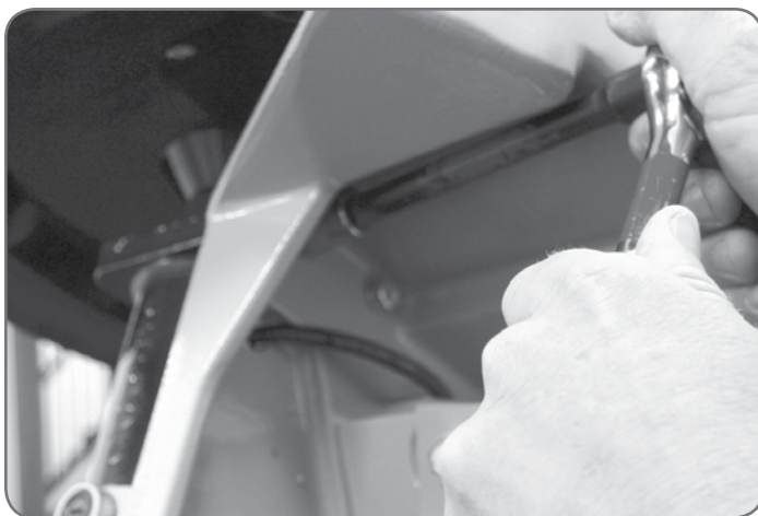
Figure 9 Shown using a 6" extension with \frac{1}{2} " socket.
